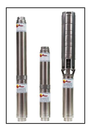
**SunPumps** SCS series submersibles are high quality, maintenance-free, DC powered pumps specifically made for water delivery in remote locations. They operate on150 to 3000 watts of DC power with voltage choices ranging from 24 to 240 volts.
