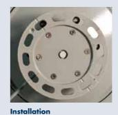
The bottom plate of the LED 350 supports installation on structure using 3 x M12 bolts or 4 x M12 bolts on a 200 mm radius. The mounting holes are galvanic isolated with plastic isolators. PTFE breathing vent for pressure release.
