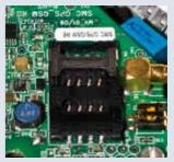
**GSM** GSM unit and antenna integra ted in the lantern for remote monitoring and control. For more
